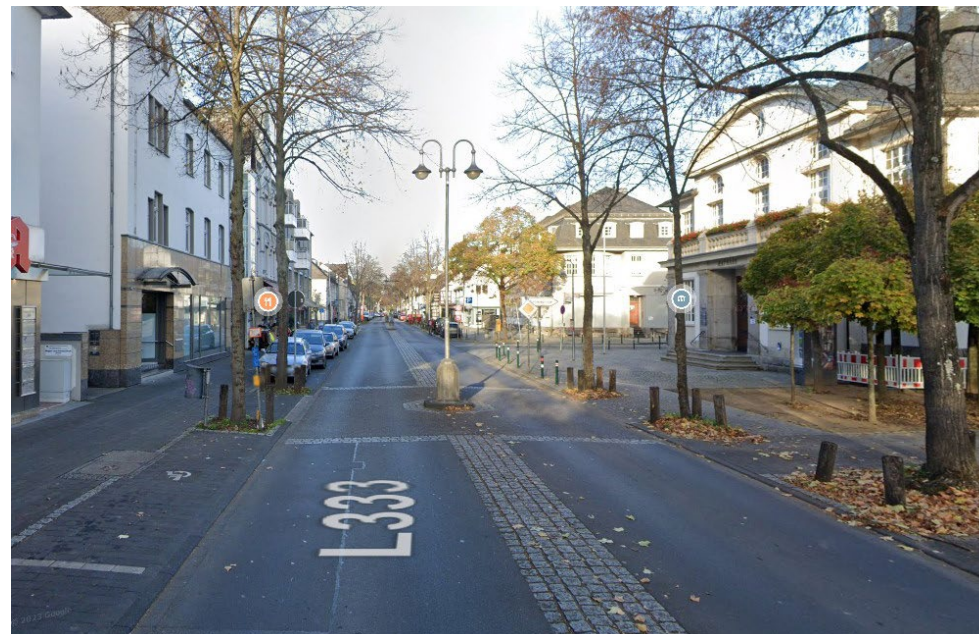
Hennef Germany - flush median used on main street
