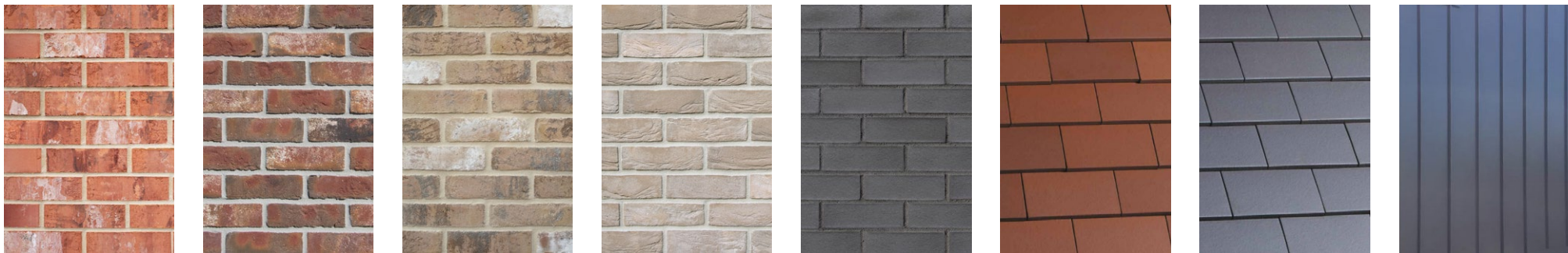
ID.XX Bricks based on the palette found across Rugby. There are many shades within each of the red, buff and dark brick palettes that could be utilised. Generally reds should be soft in texture and hue, whether light or dark. Buff-type bricks should be on the light and grey side, rather than yellow. Both should feature some variegation. Blue/black bricks should feature. Mortar choice also makes a significant impact on the way a brick appears and mortar proposals should be provided as part of material proposals.
