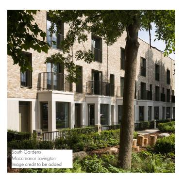
Stepping of facade and use of roof forms to distinguish individual building parts
