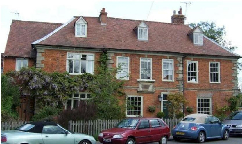
The almshouses are smaller in scale with a plainer formal style. The front elevation has a balanced layout of entrances and windows comprising Flemish bond using buff brick with a brick dentil cornice. The heavy chimneys accentuate the terraces smaller scale. Local stone has been used for sills and lintels.
